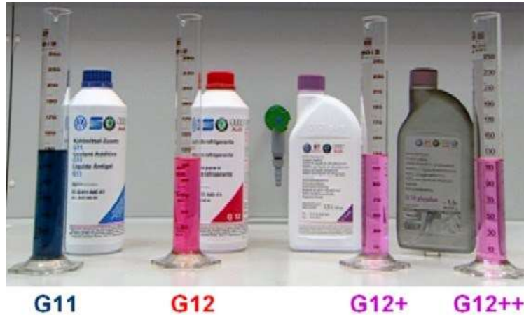
Figure 1. The color of each type of engine coolant. G11 (green-blue), G12 (red), G12+, G12++, G12evo, and G13 (purple).
