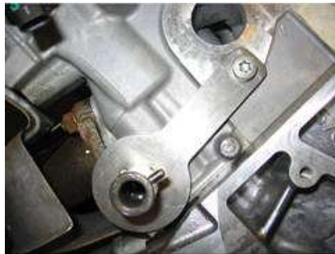
Figure 13. Engine adaptor on bank one.
