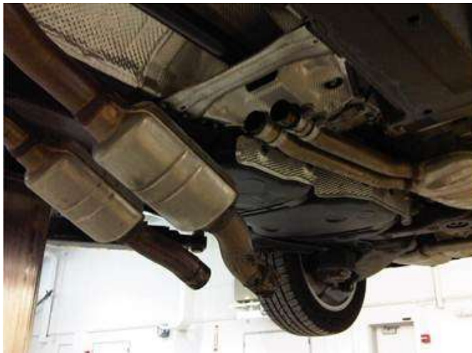
Figure 7. Lowered catalytic converter pipes.
