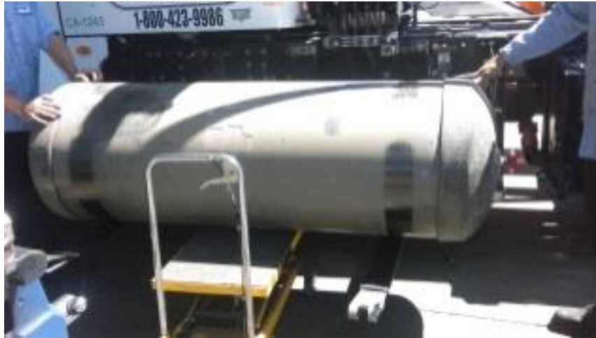
Figure 6. Cylinder being removed from the chassis.
