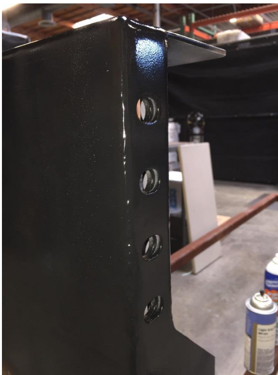
Figure 11. The bracket welded in place and painted.
