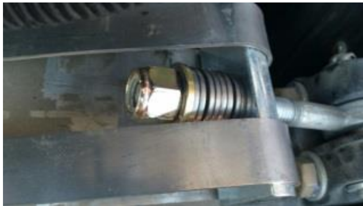
Figure 5. Belleville washer stack on the cylinder strap mounting bolts.
