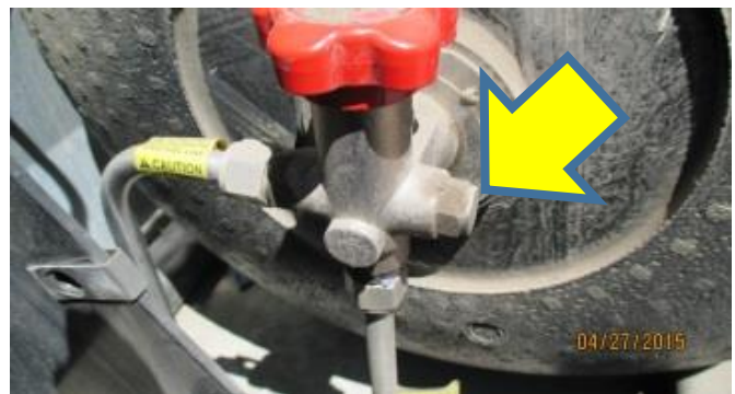
Figure 3. Two views of the plug to be removed from the cylinder valve.
