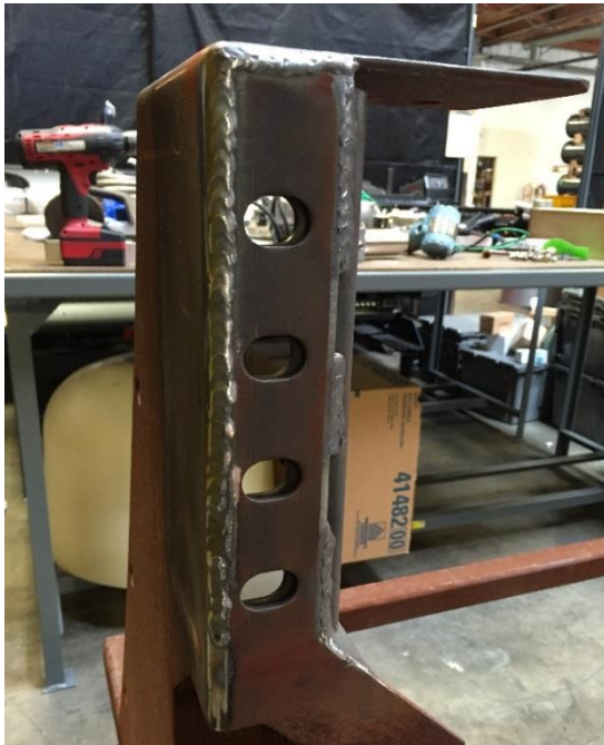
Figure 10. New bracket welded in place.
