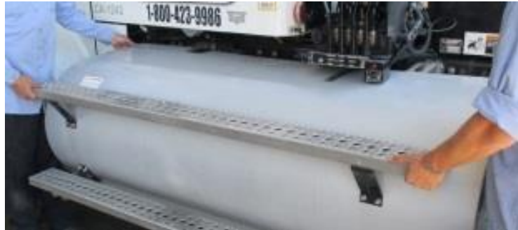
Figure 2. Lift and pull the cover and steps away from the fuel system and vehicle chassis. Use proper lifting techniques to avoid injury.
