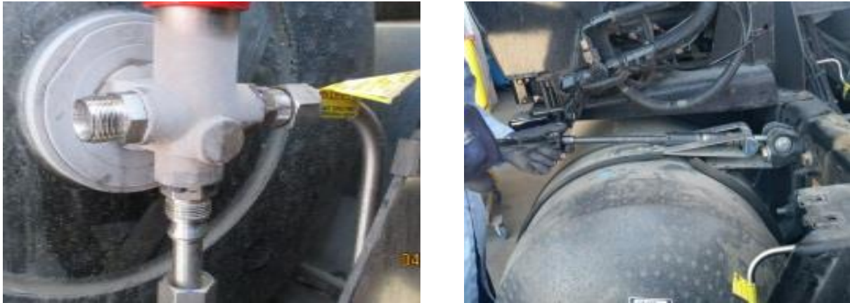
Figure 12. Left: Make sure the valve is vertical, with the handle at the 12 o'clock position. Right: A long extension bar is needed to tighten the strap bolts. Torque to 60 Ft-Lbs.
