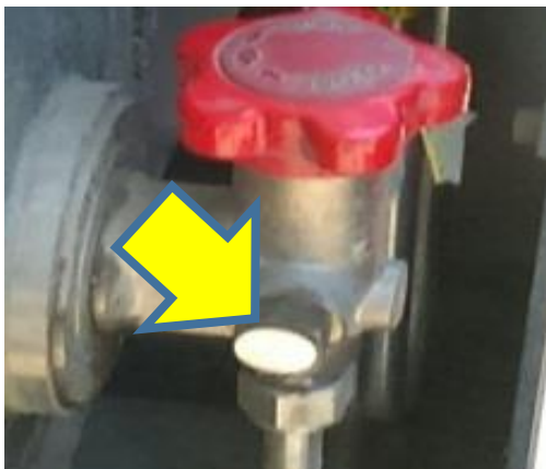
Figure 3. Two views of the plug to be removed from the cylinder valve.
