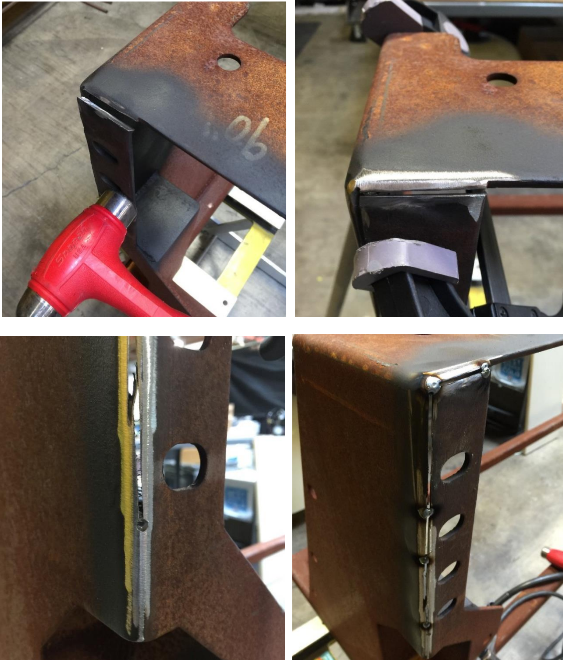
Figure 9. Tack the reinforcement plate into place. Hammer to fit as needed.
