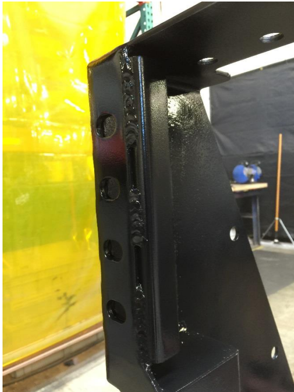
Figure 11. The bracket welded in place and painted.
