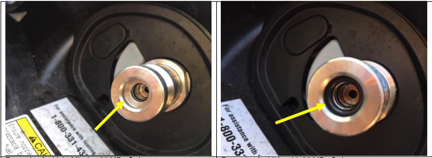
Example of vehicle Missing 35 MPa O-ring
