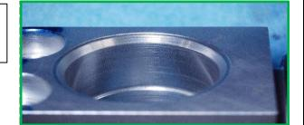
Damage - No Good Part Expansion valve seal bore is damaged due to deep scratching perpendicular to O-ring groove.
