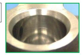
Damage – **No Good Part** Compressor seal bore is damaged due to deep scratching perpendicular to O-ring groove.
