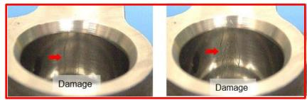
Foreign Material – **OK Part** Compressor has foreign material stuck to seal bore.
