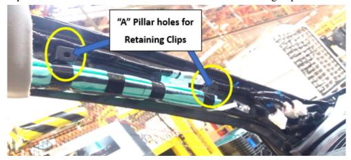
**CRITICAL:** After the 2 new retaining clips are installed onto the trim panel and before installation, confirm all side curtain airbag material is clear of the area around the "A" Pillar center hole where **Clip "B"** fits into.
