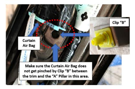
• Reinstall the "A" Pillar trim; bottom 2 trim tabs first, top Tether Clip second then **Clip "B"** into the "A" Pillar center hole. If necessary, move the trim panel around a bit to be sure both clips are started in their holes before pushing on the trim panel firmly to lock them in place.
