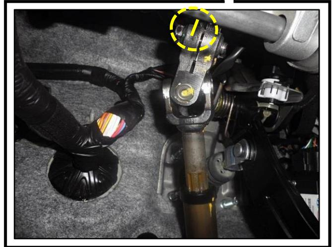
2. Prior to starting the MDPS effort measurement test (page 3), position the steering wheel slightly to the right, as shown, with the Steering Angle Sensor (SAS) in the positive range. **NOTE: attempting to start the steering effort test with the SAS in the negative range will trigger an error message and prevent the test from running.**
