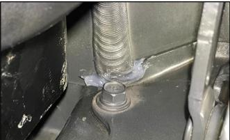
9. Continue the ¼ inch bead of the provided sealant at the gap between the factory seam sealer (H) and fender, as shown. Ensure the gap is completely covered.
