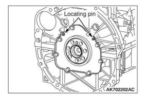
5. Install the rear oil seal case aligned with the locating pin and tighten it to the specified torque. <a href="https://example.com/ncorrect">Install the rear oil seal case aligned with the locating pin and tighten it to the specified torque.</a>
