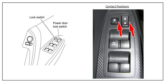
This TSB instructs dealers how to modify the taping of the branch harness to reduce the stiffness and allow more flexibility, reducing the risk of the buttons contacting the panel and sticking.
