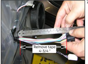
7. Remove the black tape of the harness down to 4-3/4 inches (120 mm) from the edge of the connector, as shown.
