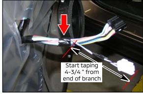
8. Tape the branch extending to the door lock switch.
