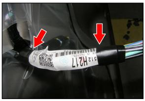
10. Reuse and attach the original part number label, taping the ends of the label as shown.
