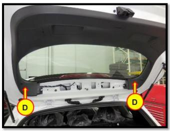
5. Using a trim tool or by hand, separate the driver side tailgate frame side trim (D).
