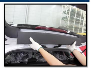
4. To remove the driver and passenger tailgate frame side trim (D), follow the below procedure.
