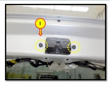
12. Remove the latch assembly (J) from the tailgate frame and set aside.
