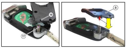
18. Turn the internal shell (8) counter clockwise until shell matches with the front shell
