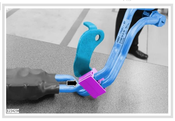
Remove the bracket from the **NEW** Transmission fluid cooler pipes (T4A29688).
