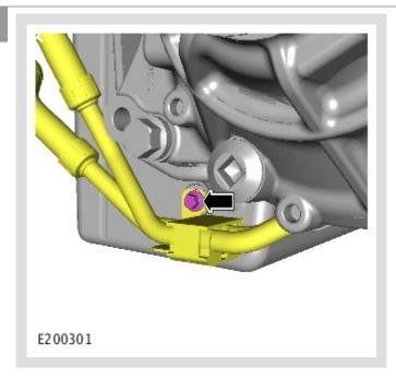
Install the bolt securing the transmission fluid cooler pipes to the oil pan.
