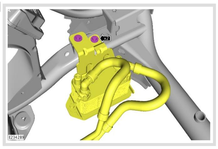
Install the transmission fluid cooler assembly to the front subframe.
