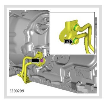
Release the transmission fluid cooler pipes.
