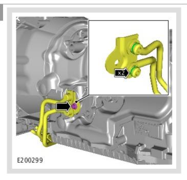
Install the transmission fluid cooler pipes.
