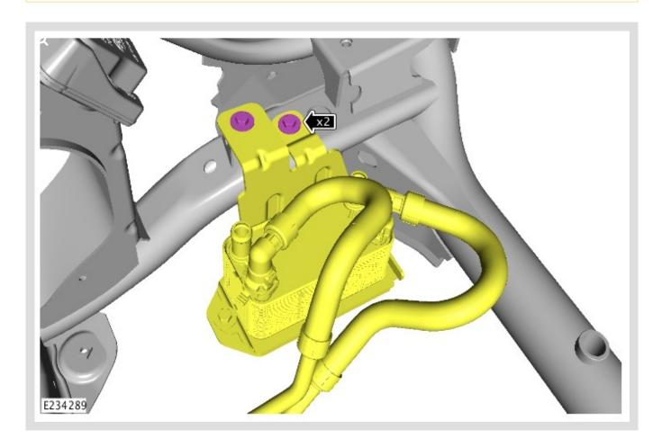
Release the transmission fluid cooler assembly from the front subframe.
