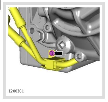
Remove the bolt securing the transmission fluid cooler pipes to the oil pan.
