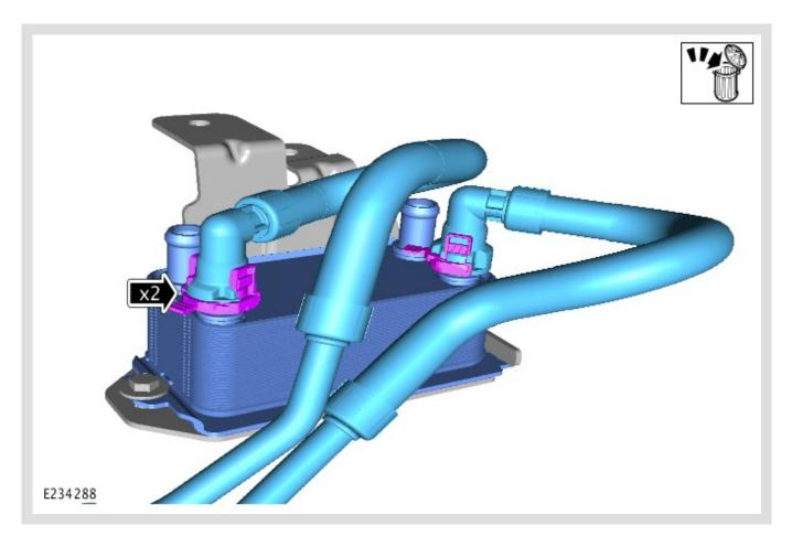
Remove and discard the transmission fluid cooler pipes.
