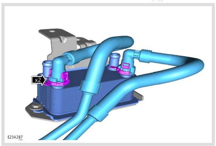
Install the new transmission fluid cooler pipes to the transmission fluid cooler.
