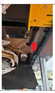
4. Using a 12mm drill bit or step bit, drill a hole through the plastic body plugs in the areas shown on the right and left sides of the vehicle.
