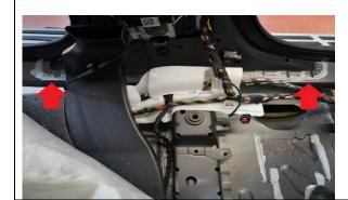
23. Using seam sealer **PN 83 42 2 409 985,** seal around the base of the B-Pillar where the B-Pillar meets the rocker panel.
