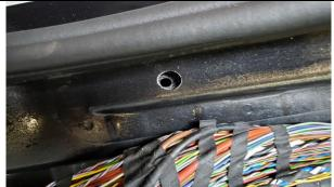
20. When step 19 is complete, the top 2 outer-most holes need to be expanded using a 12mm drill bit.
