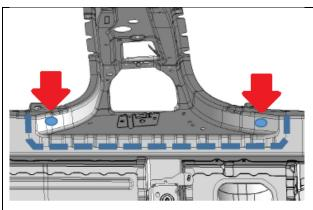
19. Using drill bit **PN 83 19 2 359 262**, drill 2 holes in the base of the B-Pillar at the locations shown by the red arrows to the left.
