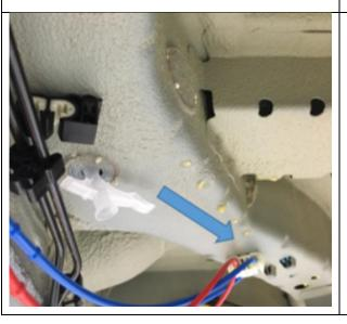
7. Using the holes that were drilled in step 4, insert the cavity foam nozzle PN 83 42 9 410 694 as far into the rail cavity as possible, facing towards the front center area of the vehicle as indicated by the blue arrow. Inject cavity foam for 3 seconds per hole. Immediately install a 12mm blind plug PN 07 14 7 127 539 into each hole.
