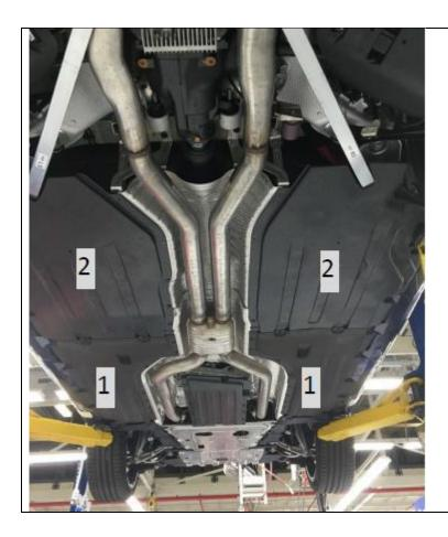
Remove the underbody panels (1 & 2) from both sides of the vehicle, following repair instructions REP 51 71 017 "Remove and install/replace left underbody paneling".
