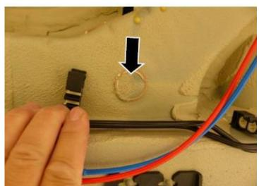
3. In the areas shown to the left, relocate and secure any lines, wires, or hoses away from the work area of the body plugs to prepare the plugs to be drilled.
