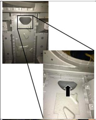
17. Coat the inside of the subwoofer cavity using cavity protection spray PN 83 42 2 457 337.
