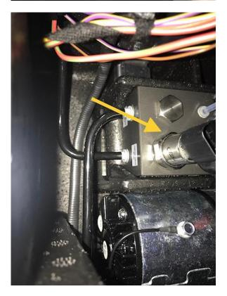
Disconnect the valve block harness and detach from foam housing
