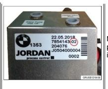
Note: The water injection valve block has been redesigned. The part number has not been changed but the optimized part can be identified by the "-02" revision index.
