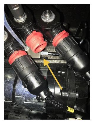
11. Disconnect the Valve 2 connector to gain access to the water pump outlet line on the valve block, disconnect the line
