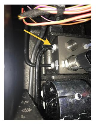
8. Disconnect the water pump inlet line from the valve block
