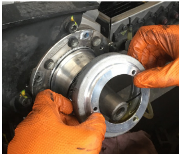
FIGURE 21: REMOVING OIL CHAMBER
