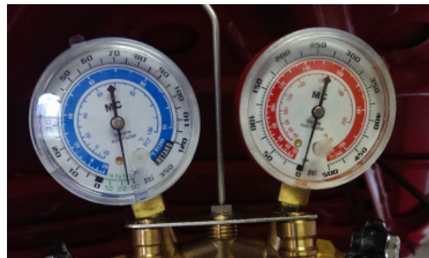
FIGURE 62: 30PSI VACUUM READING
