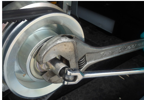
FIGURE 13: REMOVE M12 BOLT
