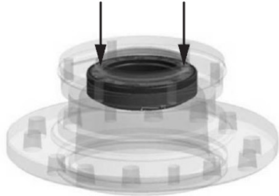
FIGURE 26: STATIONARY RING REMOVAL
