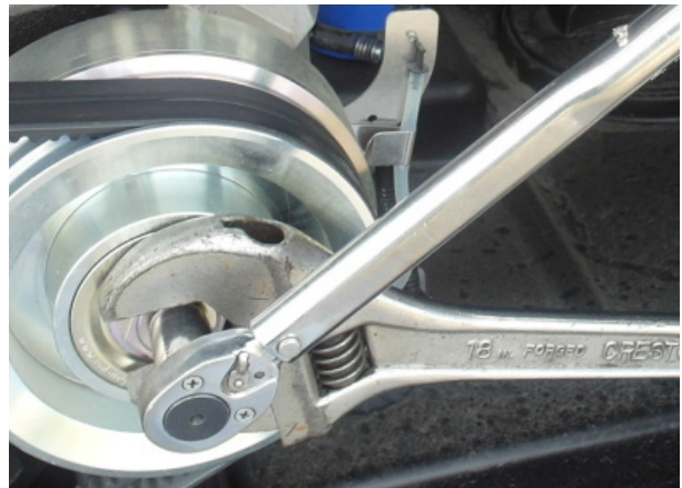
FIGURE 50: CLUTCH HOLD DOWN BOLT
