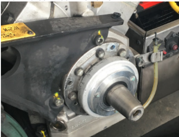
FIGURE 17: CLUTCH & COIL REMOVED
