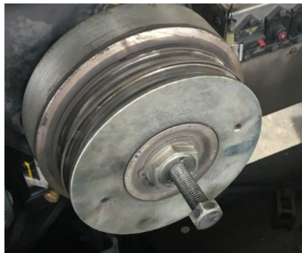
FIGURE 14: EXTRACTOR TOOL IN PLACE
