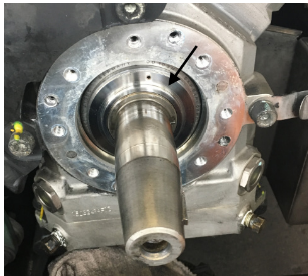
FIGURE 28: BEARING SEALING PLATE
