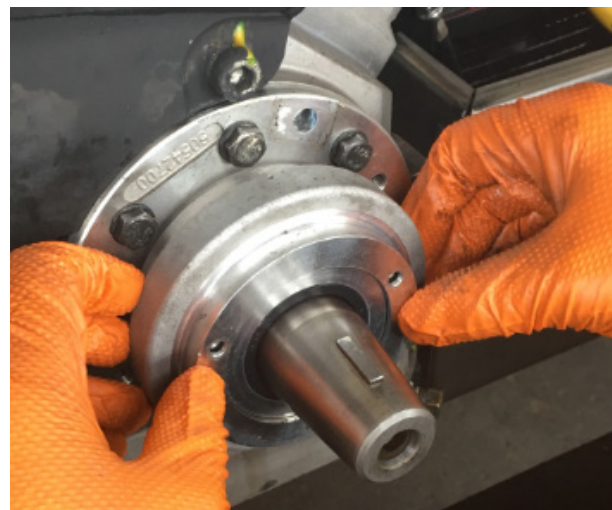
FIGURE 42: OIL CHAMBER INSTALLATION
