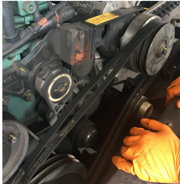
FIGURE 52: COMPRESSOR BELTS REINSTALLATION
