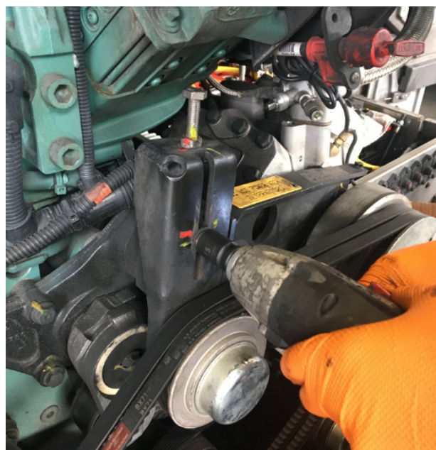
FIGURE 11: REMOVE BELT TENSIONER BOLT
