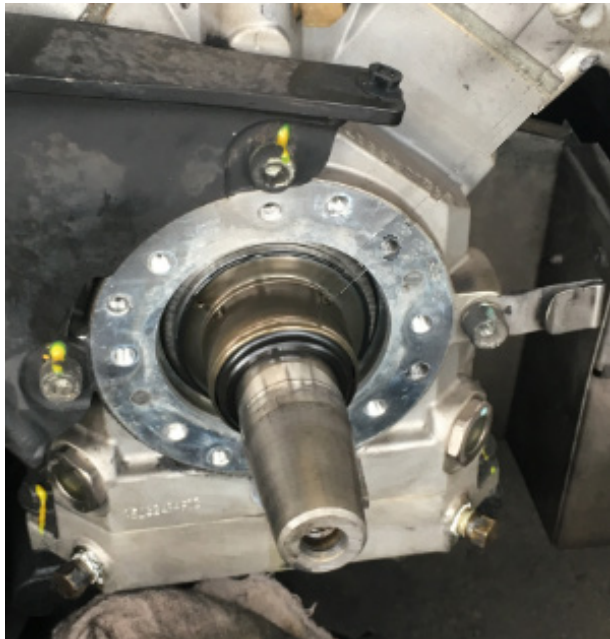
FIGURE 25: REMOVED SEALING COVER EXPOSING SLIDING RING
