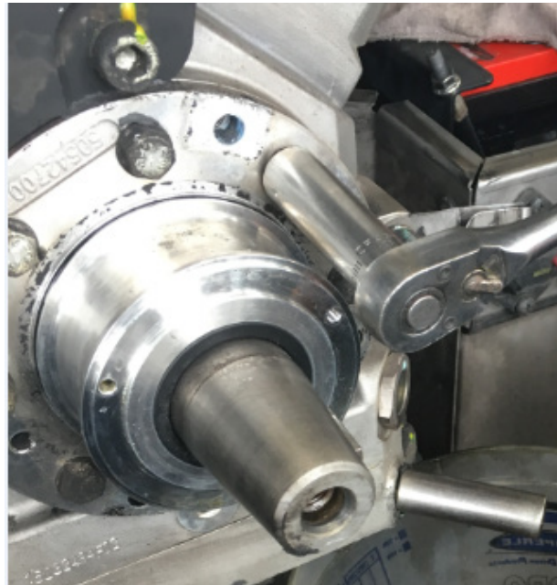
FIGURE 24: SEALING COVER REMOVAL
