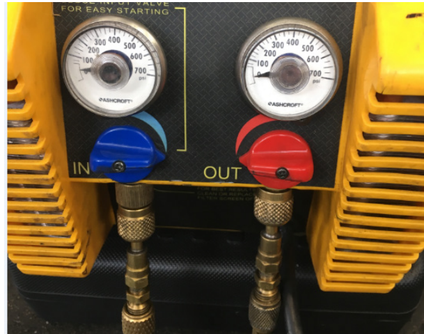
FIGURE 63: RECOVERY STATION CONNECTION
