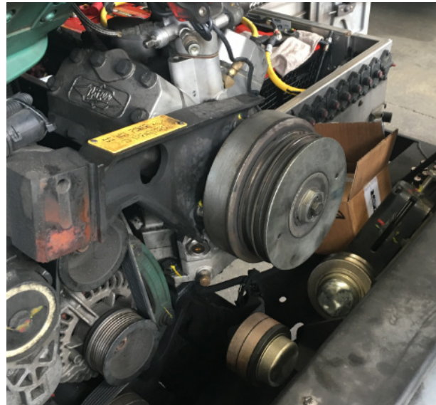
FIGURE 12: REMOVED TENSIONER & BELTS
