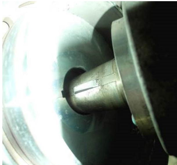
FIGURE 48: INSTALLING THE CLUTCH
