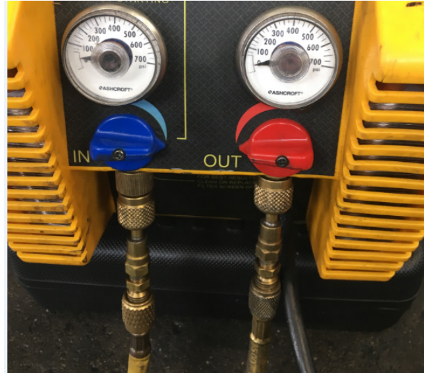
FIGURE 6: RECOVERY STATION CONNECTIONS
