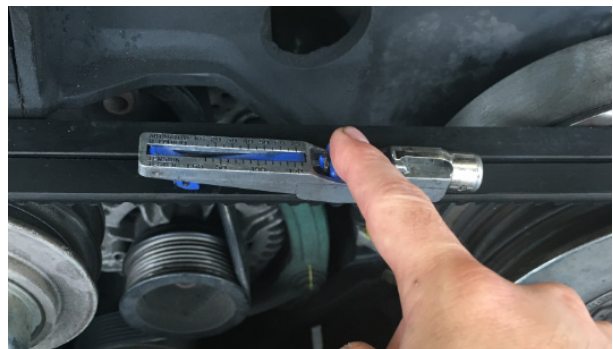
FIGURE 54: CHECKING BELT TENSION
