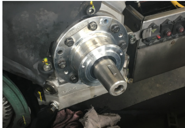
FIGURE 38: INSTALLED FRONT SEALING COVER
