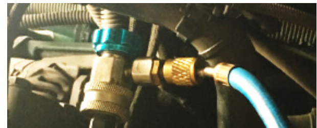
FIGURE 4: GAUGE CONNECTION (LOW PRESS. SIDE)
