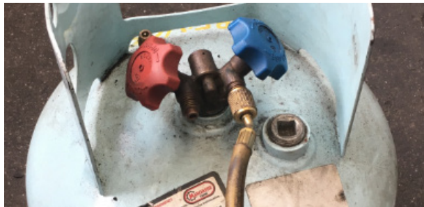
FIGURE 64: FILL TANK CONNECTION
