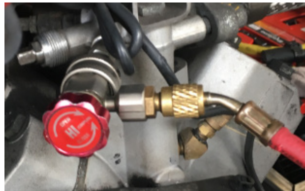
FIGURE 60: CONNECTED HIGH-PRESSURE SIDE
