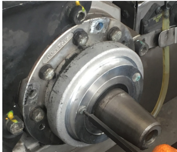
FIGURE 20: REMOVING OIL CHAMBER SCREWS
