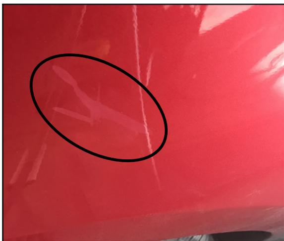
**NOTE: If there is still discoloration or blotching or a "milky" color on the paint surface after RAP-Film removal and cleaning (as shown), DO NOT REPAINT THE VEHICLE. Submit a PRC entry with photos for DPSP review, then send the vehicle to a body shop that can use an ultraviolet heat lamp to eliminate milky color spots.**
