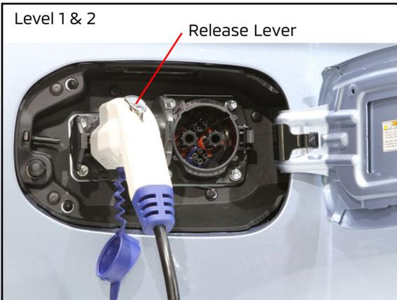
**Check proper connection of cable to vehicle.**
