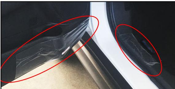
The driver entry area may be protected by a clear RAP-film placed on the scuff plate and/or lower door area. This is to protect the area from damage while the vehicle is available for viewing by customers or in dealer storage, improving Initial Quality Survey (IQS) scores.
