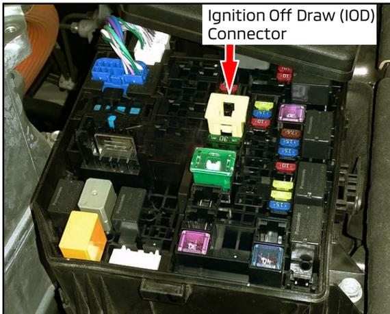
During shipping of Mitsubishi vehicles, dark current is minimized by not connecting the IOD connector. It is positioned in the disconnected position (pulled up) and must be connected by pressing it down for the affected circuits to be completed.
