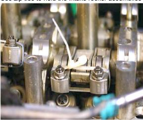
19. To prevent damage to the camshafts, loosen the bolts, in sequence, two turns at a time. Remove the camshaft holder bolts, Remove the rocker arm assembly and both cam shafts.
