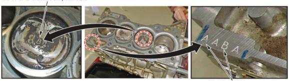
The "A" and "B" represents piston size. Piston sizes can be mixed in an engine block assembly.
