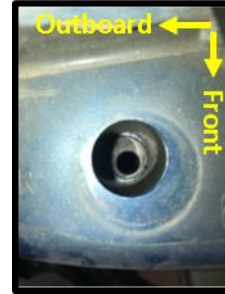
Location of Bolt top mounting surface and witness mark example
