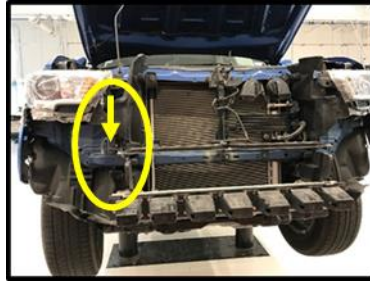
Location of Bolt top mounting surface and witness mark example
