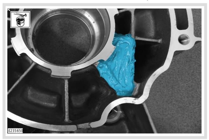
Apply an even layer of Devcon putty to the transmission insert until it is completely filled and covered.
