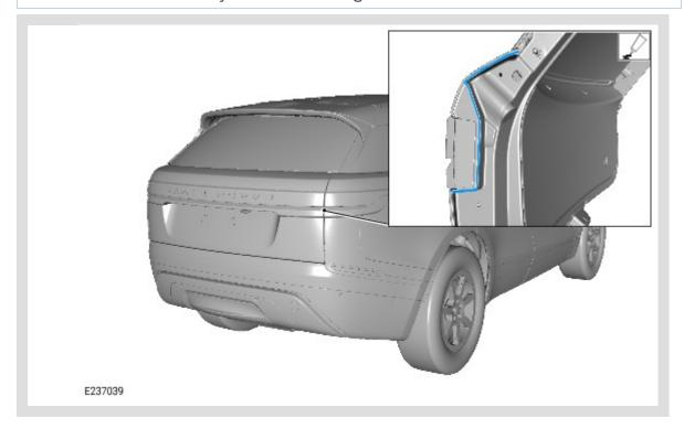
Apply sealant (Loctite® 595 or equivalent) to the tailgate in the area shown.
