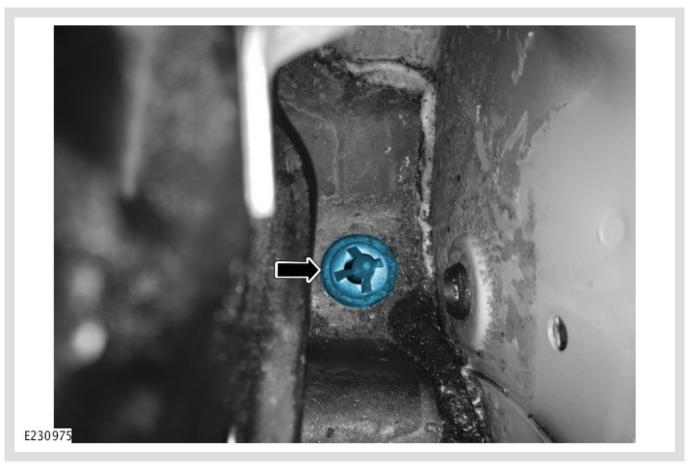
Install the drain tube stopper to the drain tube inlet.
