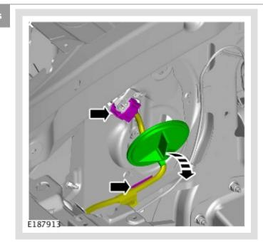
Remove the large grommet, disconnect the electrical connector, and move the wiring harness to improve access into the rear quarter panel cavity.
