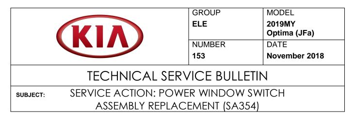
This bulletin provides the procedure to replace the main power window switch assembly on some 2019MY Optima (JFa) vehicles, produced from May 22, 2018 through August 30, 2018, which may experience a non-functioning "auto-up" window switch. Follow the procedure outlined in this bulletin to replace the main power window switch assembly.
