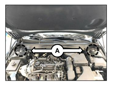
2. Remove and replace both front strut flange nuts (B) and torque the new nuts to specifications.
