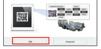
3. If the QR Reader did not successfully read the barcode, manually input the transaxle serial number (12 digits) and select **Done**. If the GDS fails to input the data, manually input the complete pressure characteristics data (72 numbers and letters). Select **OK**.
