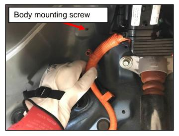
13. Remove a 10mm bolt and a 10mm nut to loosen the charging wiring harnesses.
