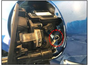
15. Use a T15 Torx screwdriver to remove the two screws holding the inlet locking actuator.
