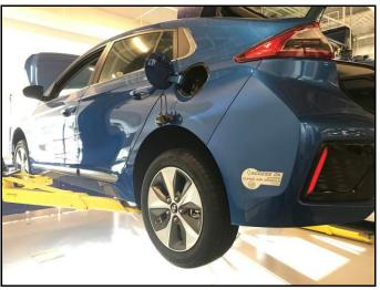
11. Remove the rear driver's side wheel by removing the 5 lug nuts.
