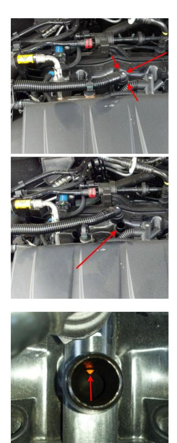
If the non return value is not visible as shown in picture, then use a long cotton swab to wipe any excess oil from the value to validate. If the non return value is still not visible, then intake manifold removal for inspection is required to validate. If the value is present reinstall the intake manifold. Do not replace.
