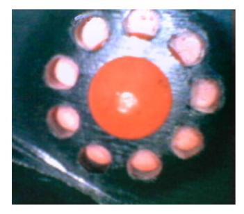
If the intake manifold Non Return Valve is missing, then replace the intake manifold assembly,
