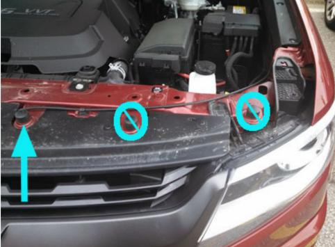
The paper test can be performed on the inner bumpers after latch adjustment. The inner bumpers should have very little to no drag to remove the paper.
