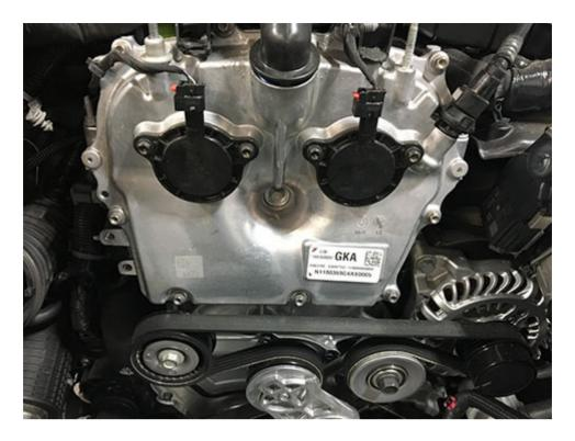
As shown in the abovephoto, the engine broadcast code can be found on the engine front cover
