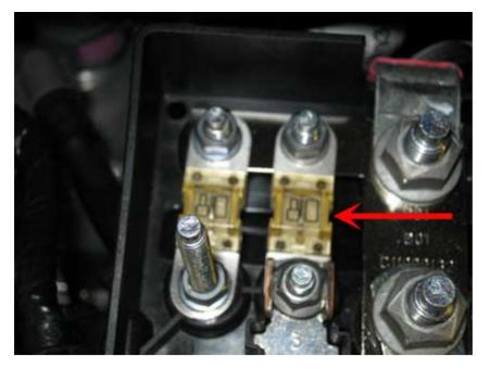
2) Check the torque on the main power feeds cable at the X50 auxiliary under hood fuse box. If loose, torque to factory spec's and retest system.
