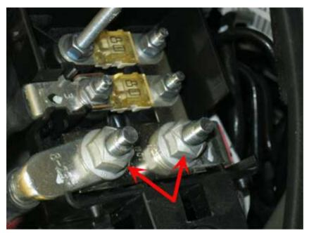
Note: You will have to remove the fuse box cover to gain access to the fuse and the main power feeds.
