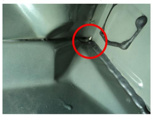
5.) Inspect for voids in the body sealer at the cowl seam on the right side under the plenum cover cap as shown in the picture below.
