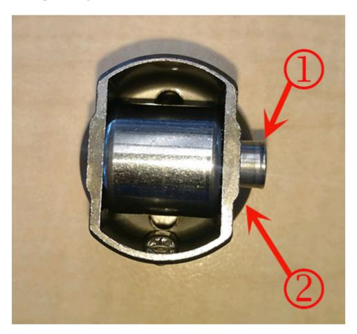
Photo below shows cylinder head bore (3) damage when pin protrudes past body of follower.
