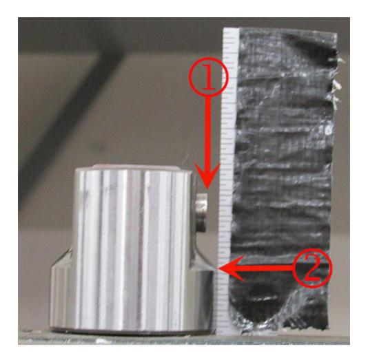
Photo below shows follower pin (1) with excessive lateral movment. Note how pin is protruding past body (2) of follower. When the "pin walk" is this excessive it will contact and damage the cylinder head follower bore.
