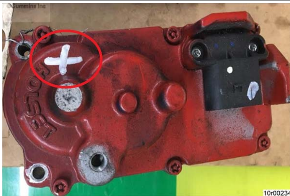
Figure 15, Witness Mark Applied.
