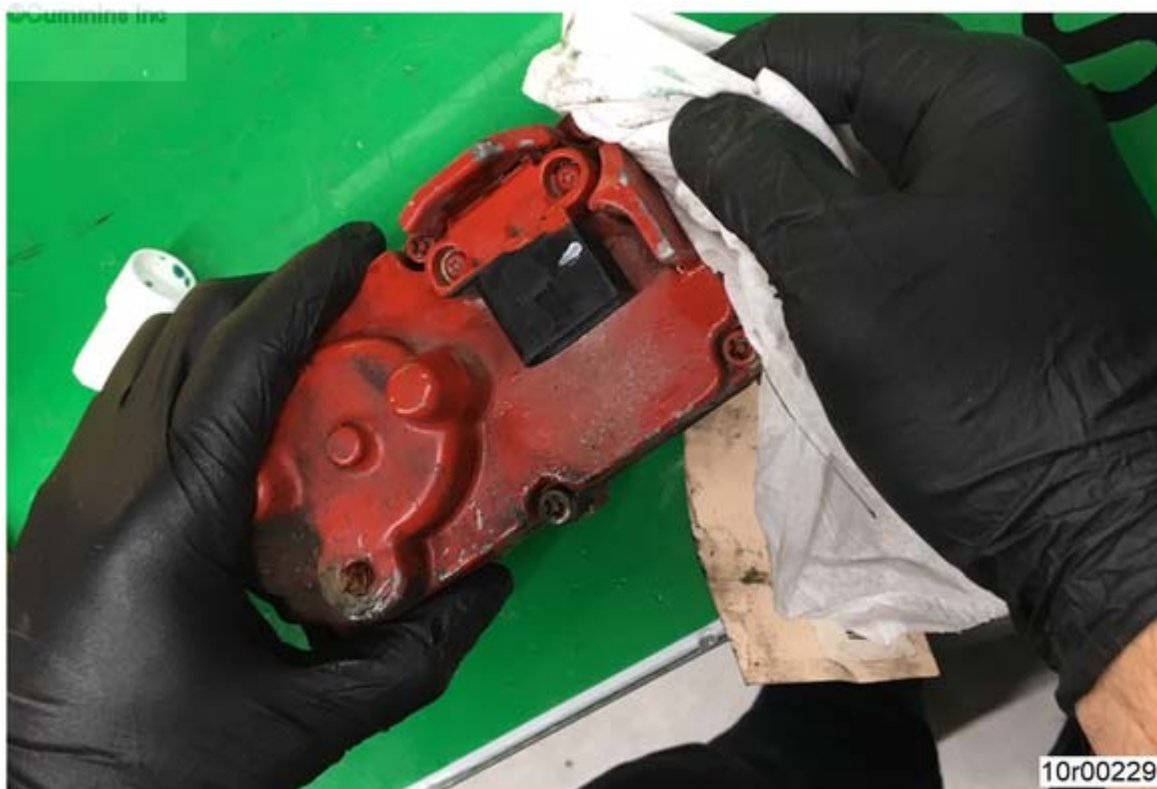
Figure 10, Cleaning Excess Loctite®.
