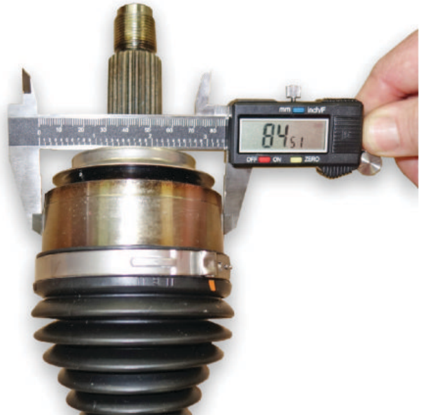
IMPROVED CV JOINT (84 mm)
