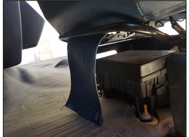
Figure 4: Flap Between Seat Adjustment Bar and Cushion
