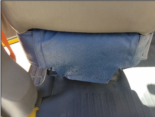
Figure 3: Flap Pulled Through Seat Cover and Seat Back then Attached with Velcro
