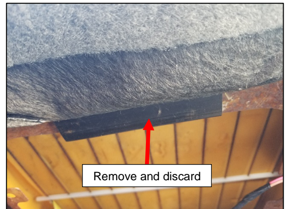
Figure 2: OEM J-hook Underneath the Rear Seat Cushion Cover
