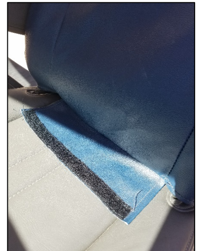
Figure 6: Seat Back Cover Flap Pulled Between the Seat and Cushion
