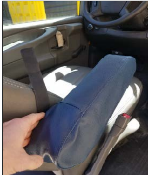
Figure 12: Tuck In the Velcro Strap
