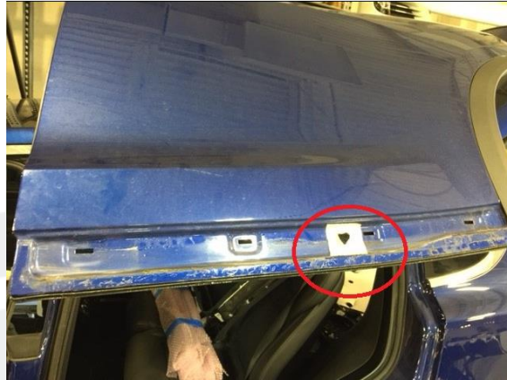
Figure 1 (Butyl patch location)
