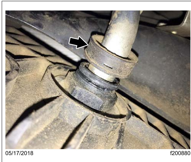
Fig. 4, Removing the Plastic Cap
