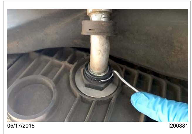
Fig. 5, Removing the Spring Clip
