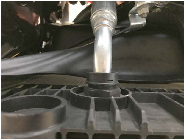
Fig. 2, Cooler Line Connection with Original Plastic Cap and Spring Clip
