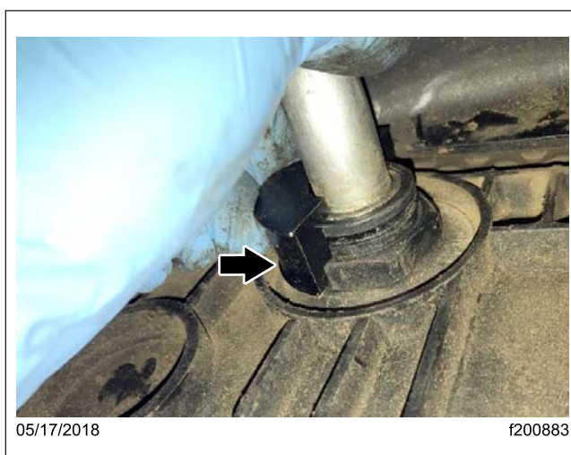
Fig. 6, Half of Collar Assembly Installed
