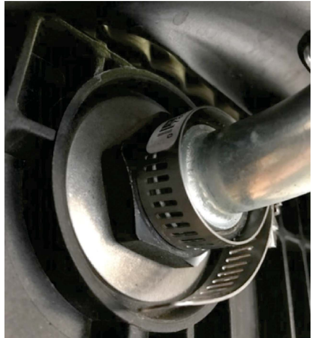
Fig. 3, Cooler Line Connection with Hose Clamp
