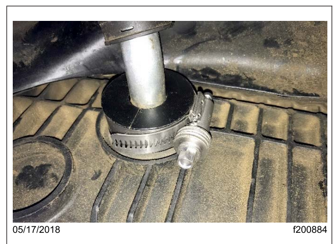
Fig. 7, Collar and Clamp Installed
