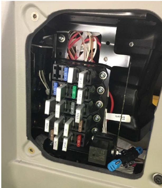
Aux PDM and location of Ground stud on Aux PDM Bracket
