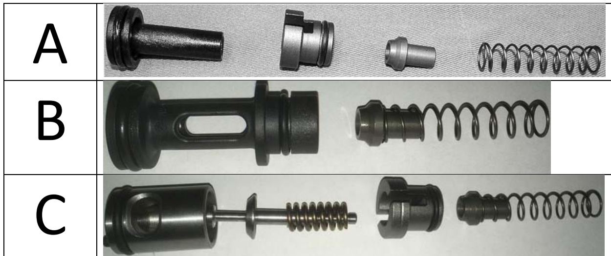
Figure 13 – Oil Pump Relief Valve
