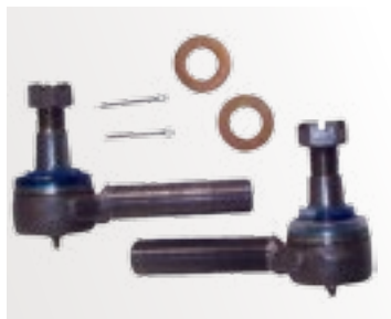
Straight Tie Rods 1 1/4" Threads, 4.25" Drop
