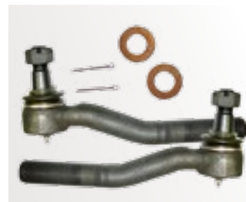
Drop Tie Rods 1 1/4" Threads, 5.36" Drop
