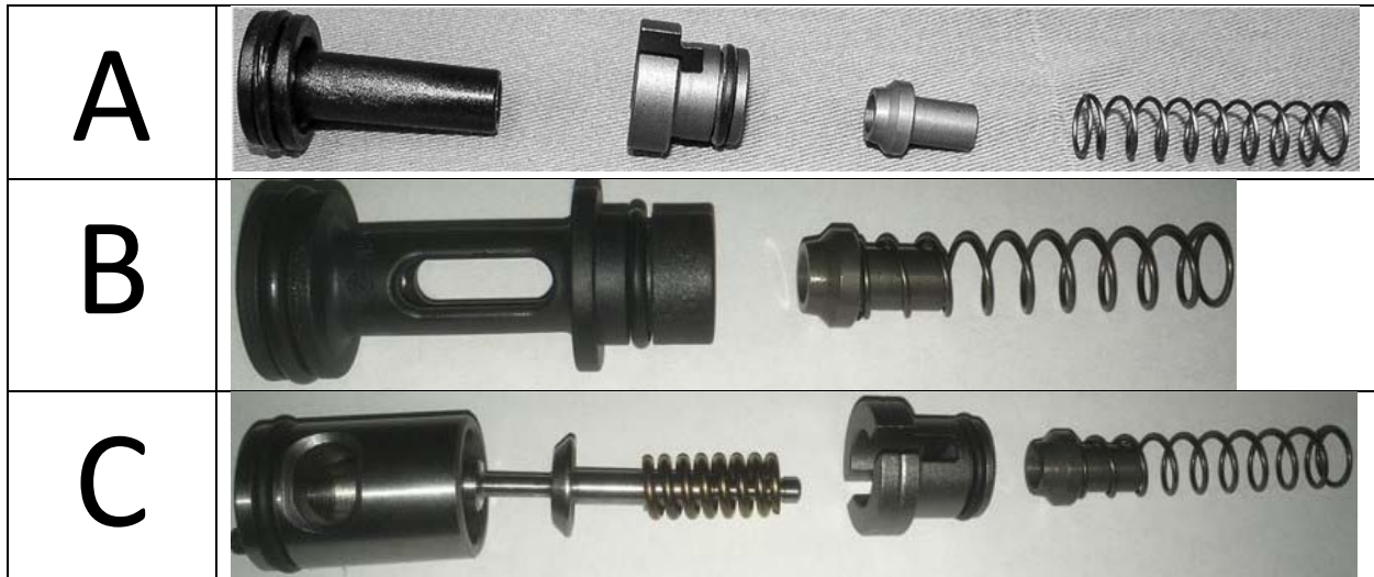
Figure 13 – Oil Pump Relief Valve
