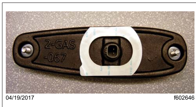
Fig. 1, Marker Light with Peel-and-Stick Adhesive Gasket
