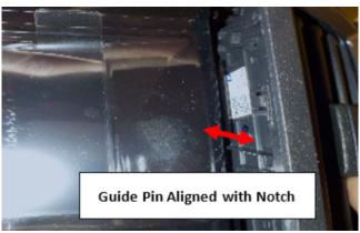
Once the vent grille assembly is in position the use both hands and press firmly down from **bottom to top** making sure it "clicks" into place. Insure there are no gaps as shown below. If the vent grille assembly still has a gap or does not feel like it is seating properly or binds as it is being installed, confirm the guide rib is properly aligned in the notch. Once alignment is confirmed, the vent grille assembly should slide into place normally.
