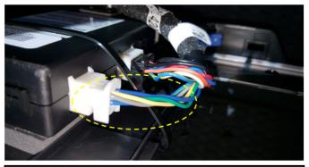
In the event of a "no-start" condition using the vehicle key, and vehicle fuse #33 (7.5A) in the main fuse box is blown, check the RES harness insulation (gray wire, pin 5 of 8-pin connector) for damage or potential short to a metal bracket. Remove and replace damaged harness if necessary.
