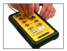
3. The tester indicates the remaining battery capacity in the LED display.
