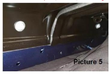
6. Place the first piece of tape 5NN 803 600 horizontally and form it to the body and the plenum chamber. Take care to not obstruct the lower holes.
