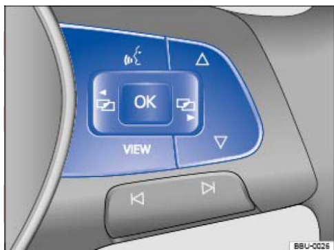
Figure 1: Right side of the multi-function steering wheel: Controls for the menus and information in the instrument cluster display.
