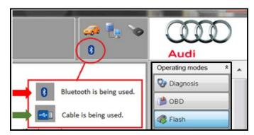
6. Using "Flash", perform the update using the SVM action code, 24DBA064.
