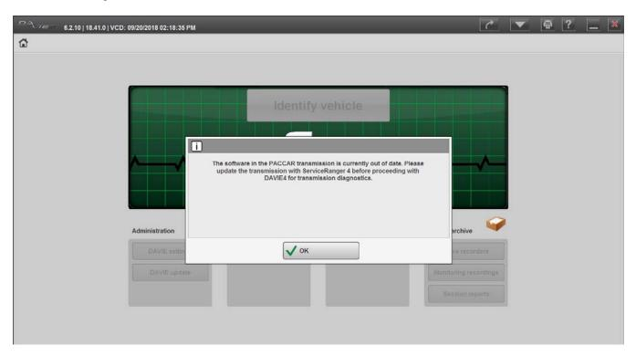
All vehicles built with PACCAR Transmissions starting October 22, 2018 and later will have the 2149629 software. If the PACCAR Transmission software level is below 2149629, ServiceRanger4 is required to apply the software update. A software change notice describing the PACCAR Transmission software changes can be found on Eportal at Service Tab / Software.
