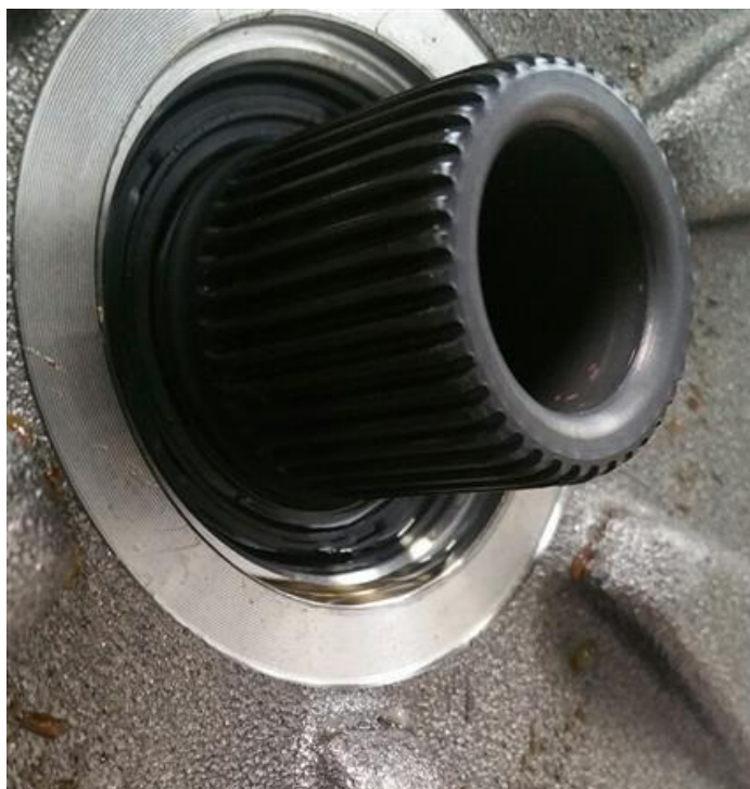
Figure 2. Oil leak at the input shaft.
